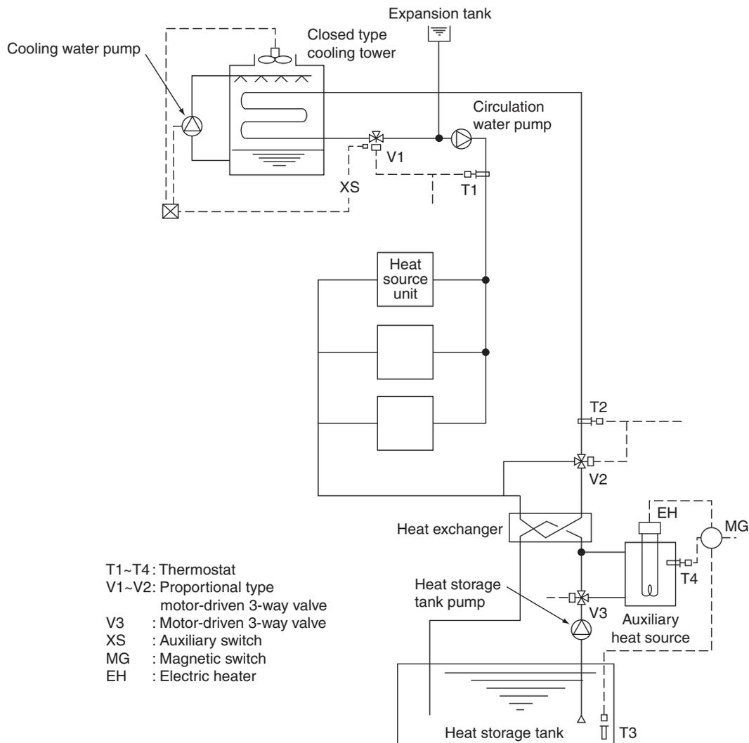
By detecting the circulation water temperature of the water heat source CITY MULTI system with T1 (around 32°C) and T2 (around 20°C), the temperature will be controlled by opening/closing V1 in the summer and V2 in the winter.
