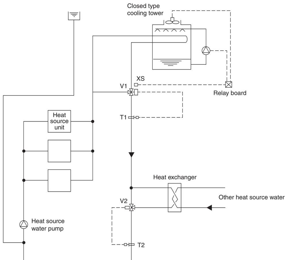
In the summer, as the circulation water temperature rises exceeding the set temperature of T1, the bypass port of V1 will close to lower the circulation water temperature. In the winter, if the circulation water temperature drops below 26°C, V2 will conduct water temperature control to keep the circulation water temperature constant.
